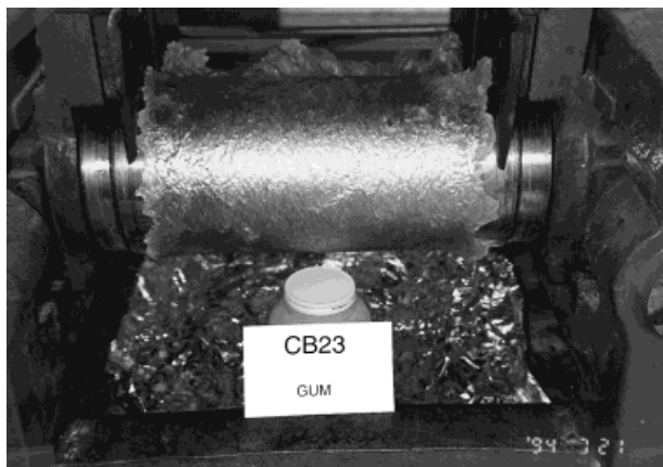
Figure 3 Photograph of CB23 gum rubber on the mill.
